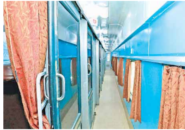
AC coaches have been provided with in-built reading lamps, insulation against noise, automatic sliding doors and auto - closing vestibule door
