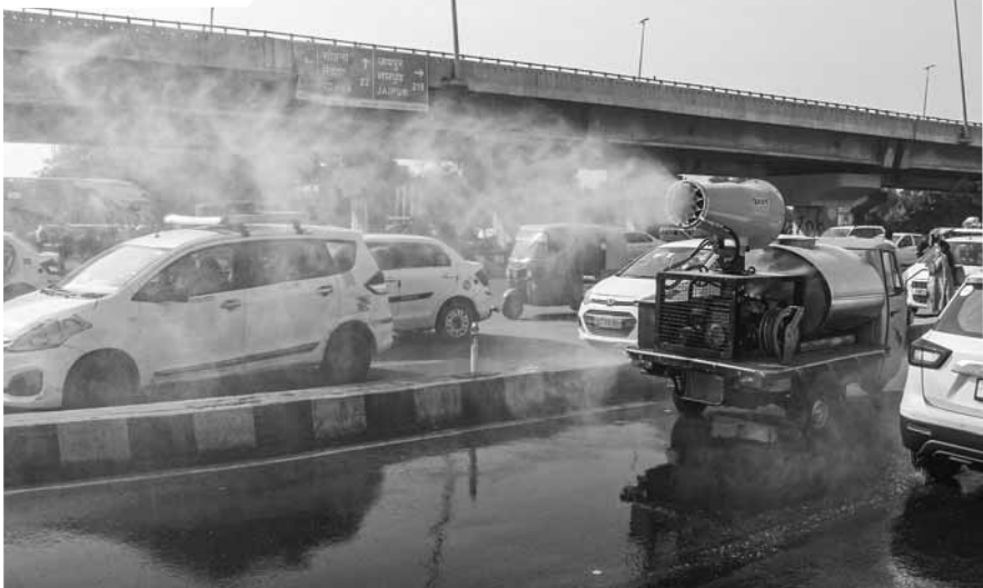
An anti-smog gun sprays water droplets to curb air pollution, in Gurugram
