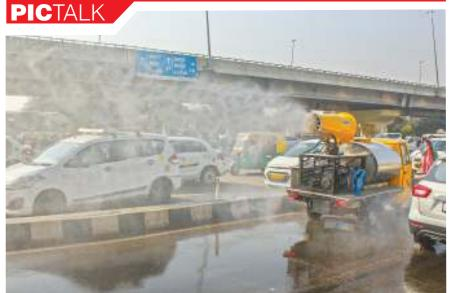
An anti-smog gun sprays water droplets to curb air pollution, in Gurugram
