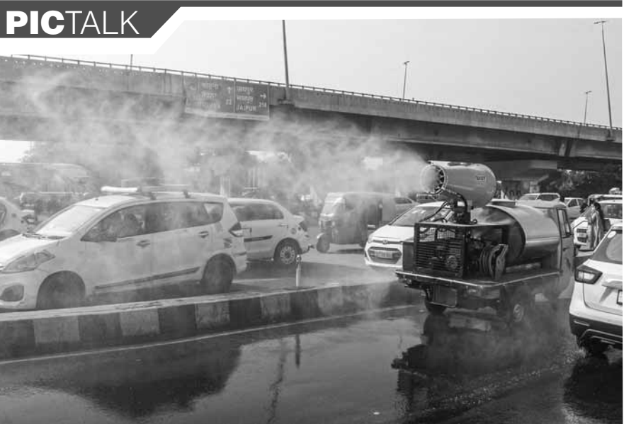
An anti-smog gun sprays water droplets to curb air pollution, in Gurugram
