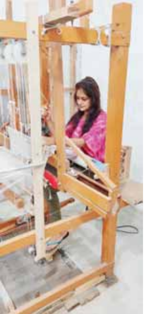
A female handloom weaver working on an ergonomically designed loom developed for handloom weavers by the Mechanical Engineering department of IIT (BHU).
