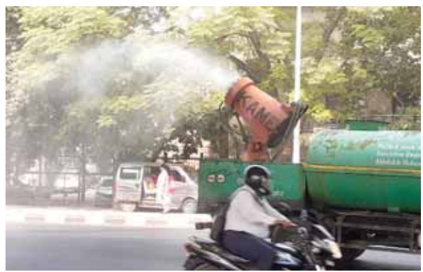
An anti-smog gun sprays water vapour to curb air pollution in Delhi on Monday
