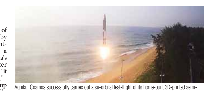
Agnikul Cosmos successfully carries out a su-orbital test-flight of its home-built 3D-printed semi-cryogenic rocket Agnibaan from its own launch pad at Sriharikota, on Thursday
