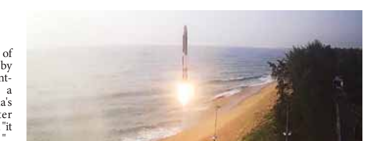
Agnikul Cosmos successfully carries out a sub-orbital test-flight of its home-built 3D-printed semi-cryogenic rocket Agnibaan from its own launch pad at Sriharikota, on Thursday
