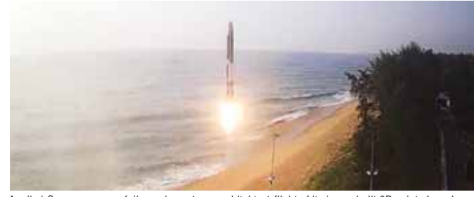
Agnikul Cosmos successfully carries out a su-orbital test-flight of its home-built 3D-printed semi-cryogenic rocket Agnibaan from its own launch pad at Sriharikota, on Thursday
